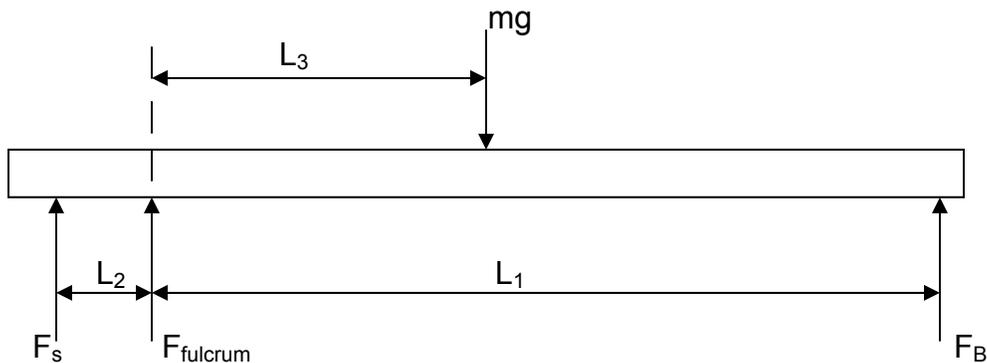
Note that only net forces are shown. For example, at the left end the counterweight is acting downwards and the scale is applying a force upwards. Since only the changes in force will be used in the analysis we can resolve the two forces as one net force  $F_s$ . Similarly, the net force resulting from the weight of the test sphere and tube, as well as the magnetic force applied by the solenoid, are resolved into  $F_B$ . A torque balance about the fulcrum yields:
