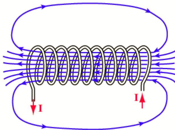
*Fig. 2: Finite Solenoid*
