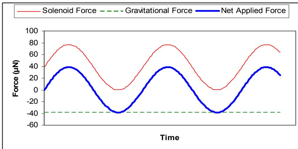
Fig. 5: Forces acting on Sphere
