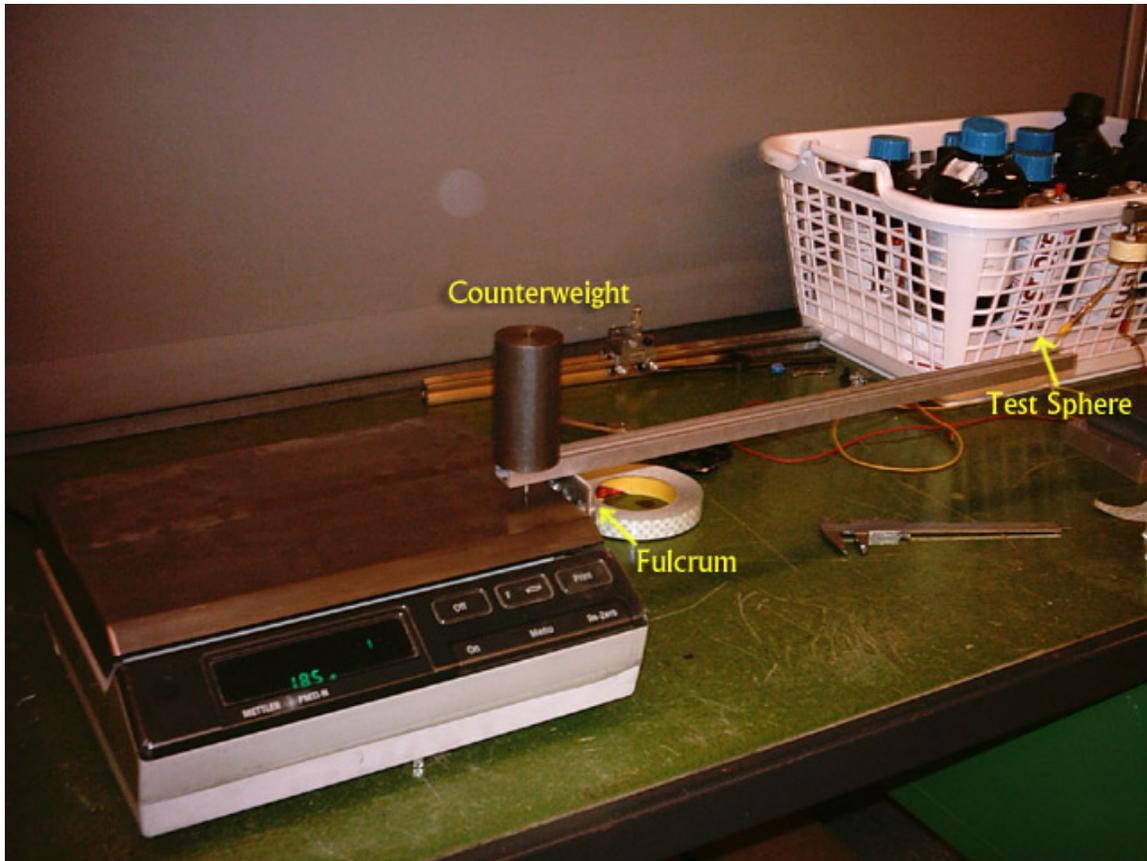
*Fig. 6: Counterbalanced Beam Scale*
